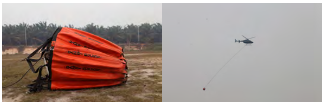
Images 5 and 6: A helicopter can carry up to 10,000 litres of water in its bucket (left) to extinguish a fire.
